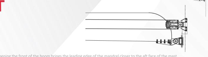
Opening the front of the boom brings the leading edge of the mandrel closer to the aft face of the mast.
