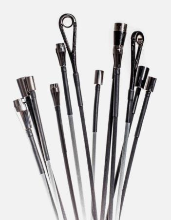
ECsix, is constructed using small, pultruded, high modulus carbon rods which are terminated either in a conical/friction style fitting or an eye style end.
